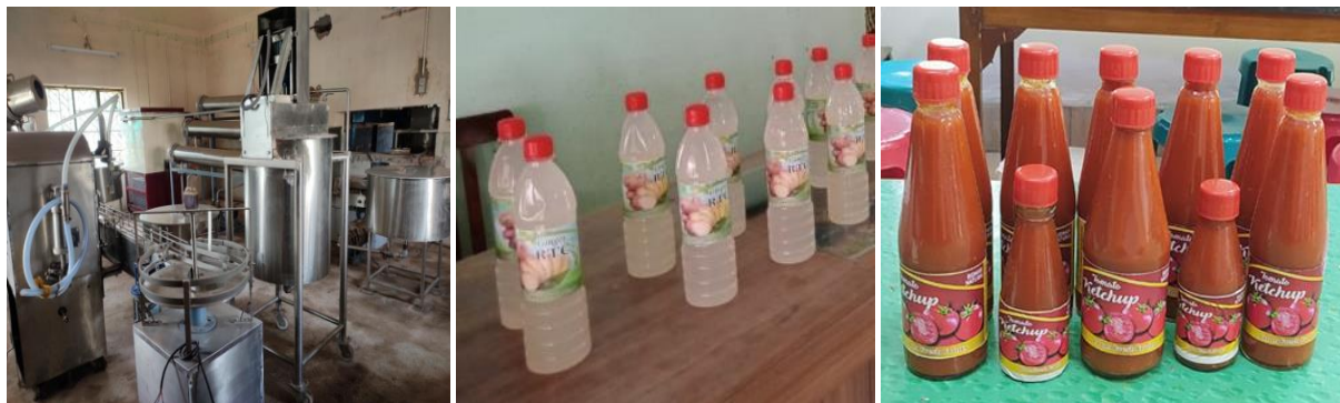
Pasteurization unit, Automatic bottle filling machine, Lime-ginger RTC and Tomato ketchup prepared by ELP students
