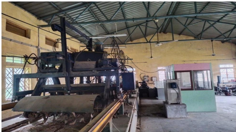
Soil Bin Set-up in Farm Machinery Testing Laboratory
