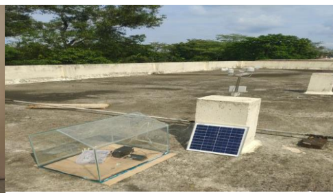
IoT-Based Weather Monitoring System (Ag. Engineering Building)
