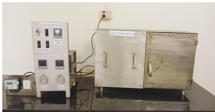
Heat Pump Drying Unit in Food Engineering Lab
